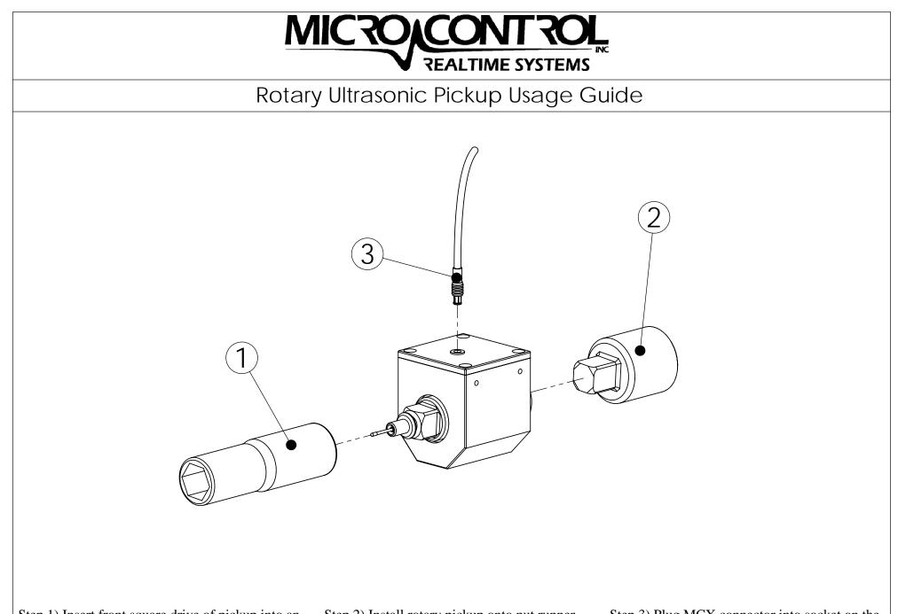
Step 1) Insert front square drive of pickup into an electrically conductive socket. Ensure probe is not damaged during procedure.
